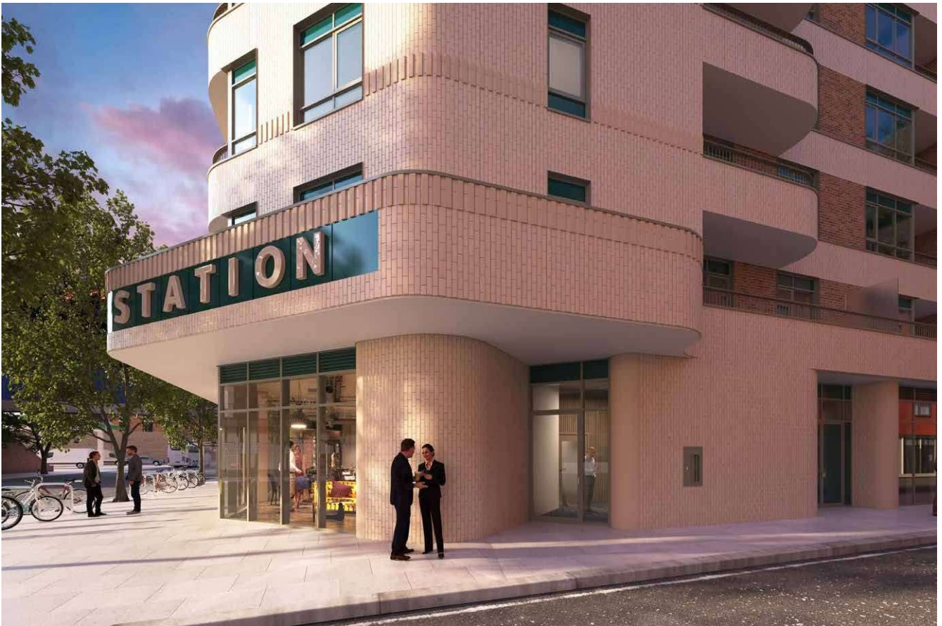
CGI image showing the vertical soldier course brickwork and projecting 'fentil' brick course at window cill and canopy cornice level
